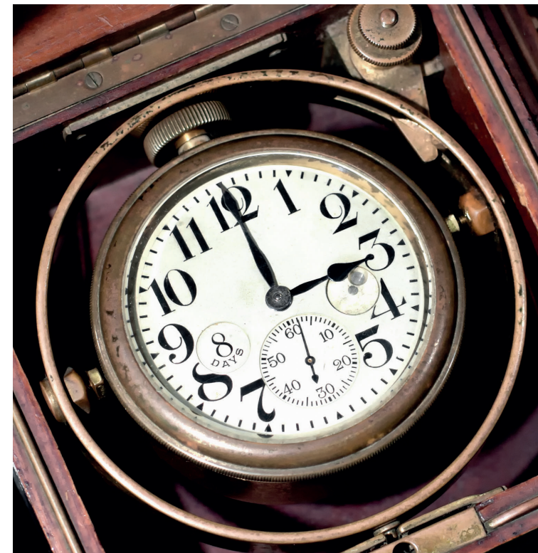
The seagoing chronometer enabled ships to ascertain longitudinal position within a ten-mile margin of error—remarkably accurate for its times.
