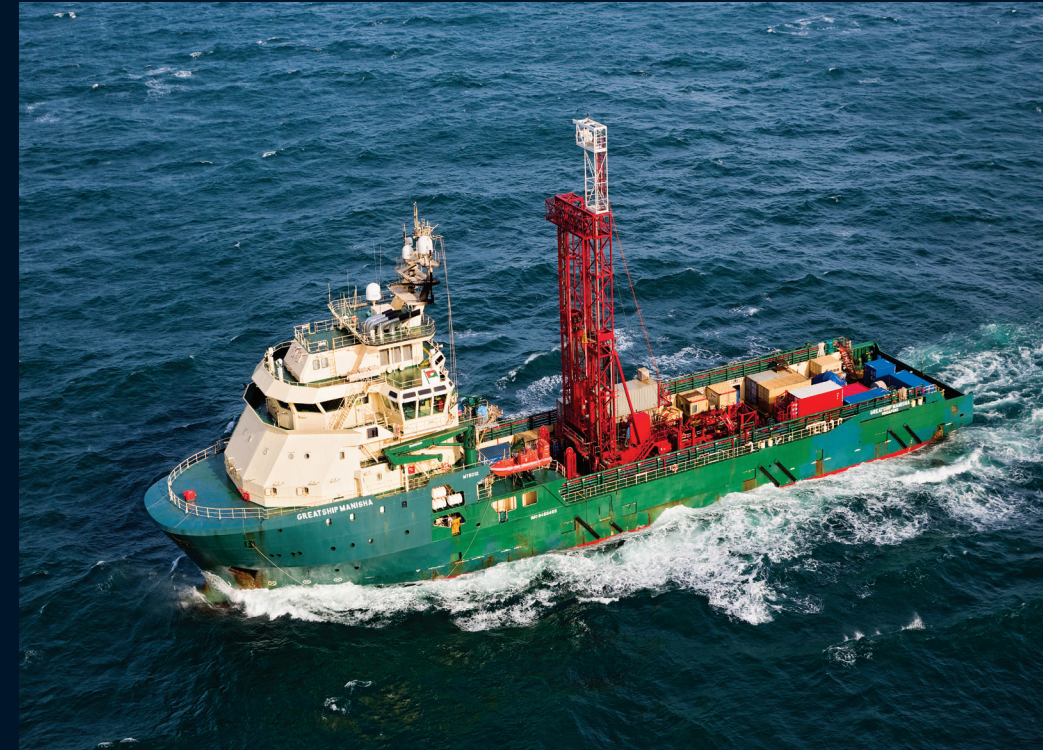
Greatship Manisha is a DP2, 4,221 dwt diesel-electric MPSSV built at Keppel Singmarine.
